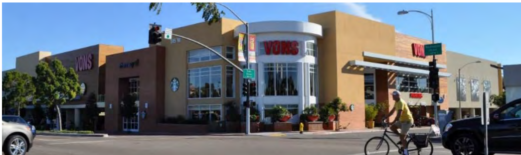
Above: A corner retail store has a well screened parking garage and features that exemplify acceptable building modulation, which include varying heights, change in color, building material, and the use of projections to provide visual interest.
