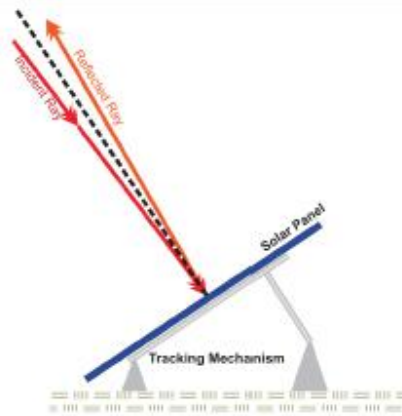
Incident and reflected rays of light that would result from an optimally oriented solar panel on a variable tilt single axis tracking mechanism.
