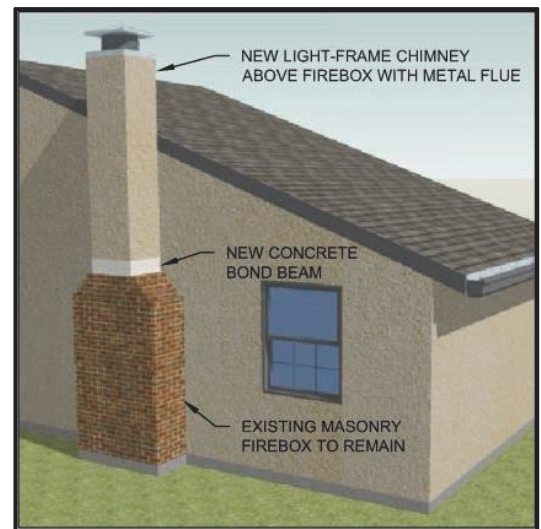
Figure 4: Dwelling with the chimney reconstructed from the firebox up
