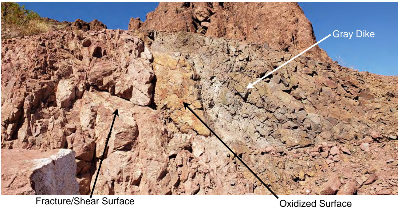
Photo 2. Closeup of existing rock quarry face viewed toward the northwest showing jointed reddish brown andesite rock material and highly fractured gray andesite dike with orange oxidized joint surface. Note localized fracture/shear surface.
