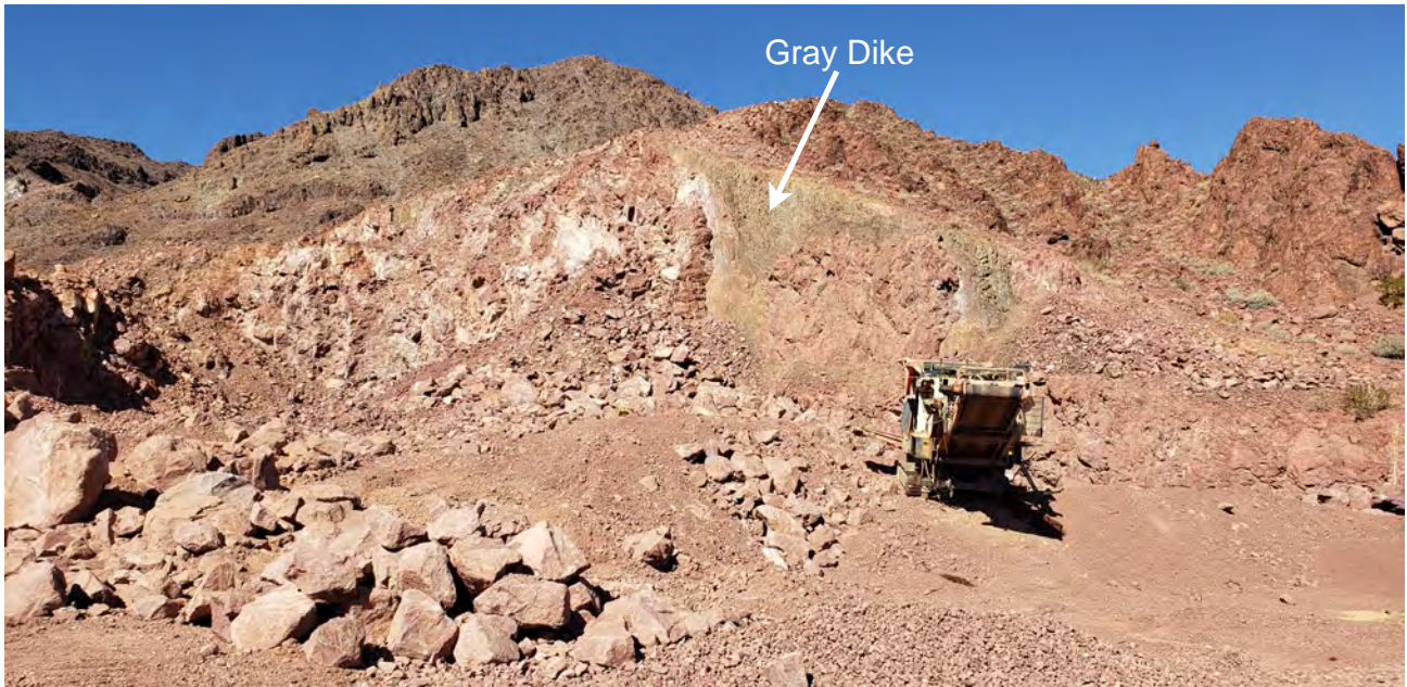
Photo 1. Existing rock quarry face viewed toward the northwest showing reddish brown andesite rock material and gray andesite dike
