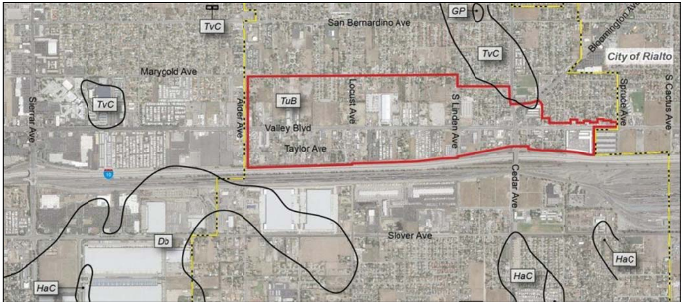
Figure 3. Soils Map. (Specific Plan area boundary in red; Db, Delhi fine sand; TuB, Tujunga loamy sand; TvC, Tujunga gravelly loam; hAc, Hanford coarse sandy loam.
