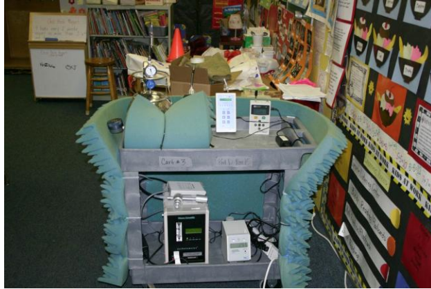
Figure 6. One of the four mobile stations used to monitor the indoor and outdoor concentrations of the targeted air pollutants
