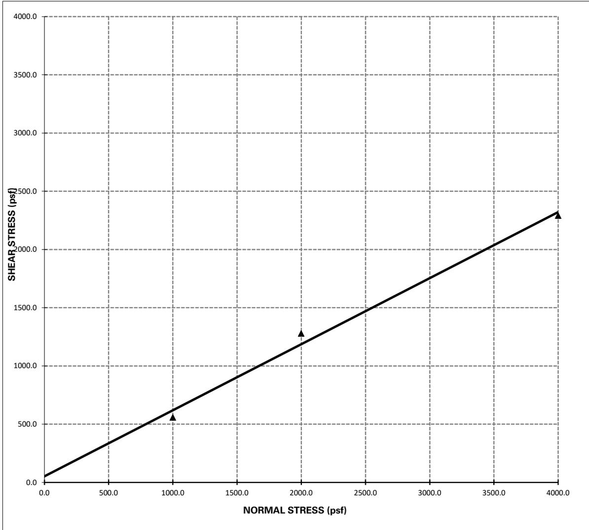
**Shear Strength:**  $\Phi = 30^\circ$ , **C = 52 psf**
