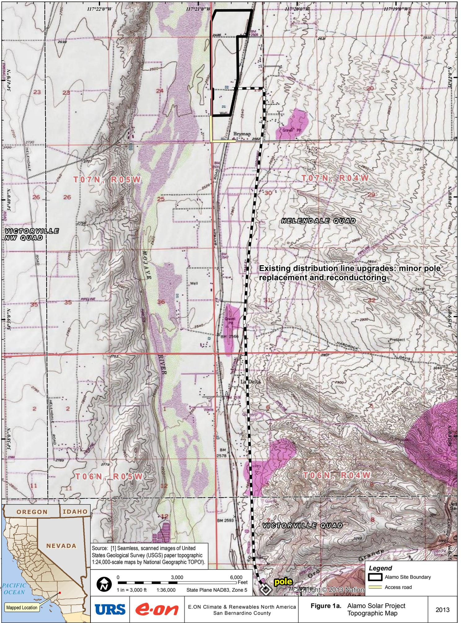
Existing distribution line upgrades: minor pole replacement and reconductoring
