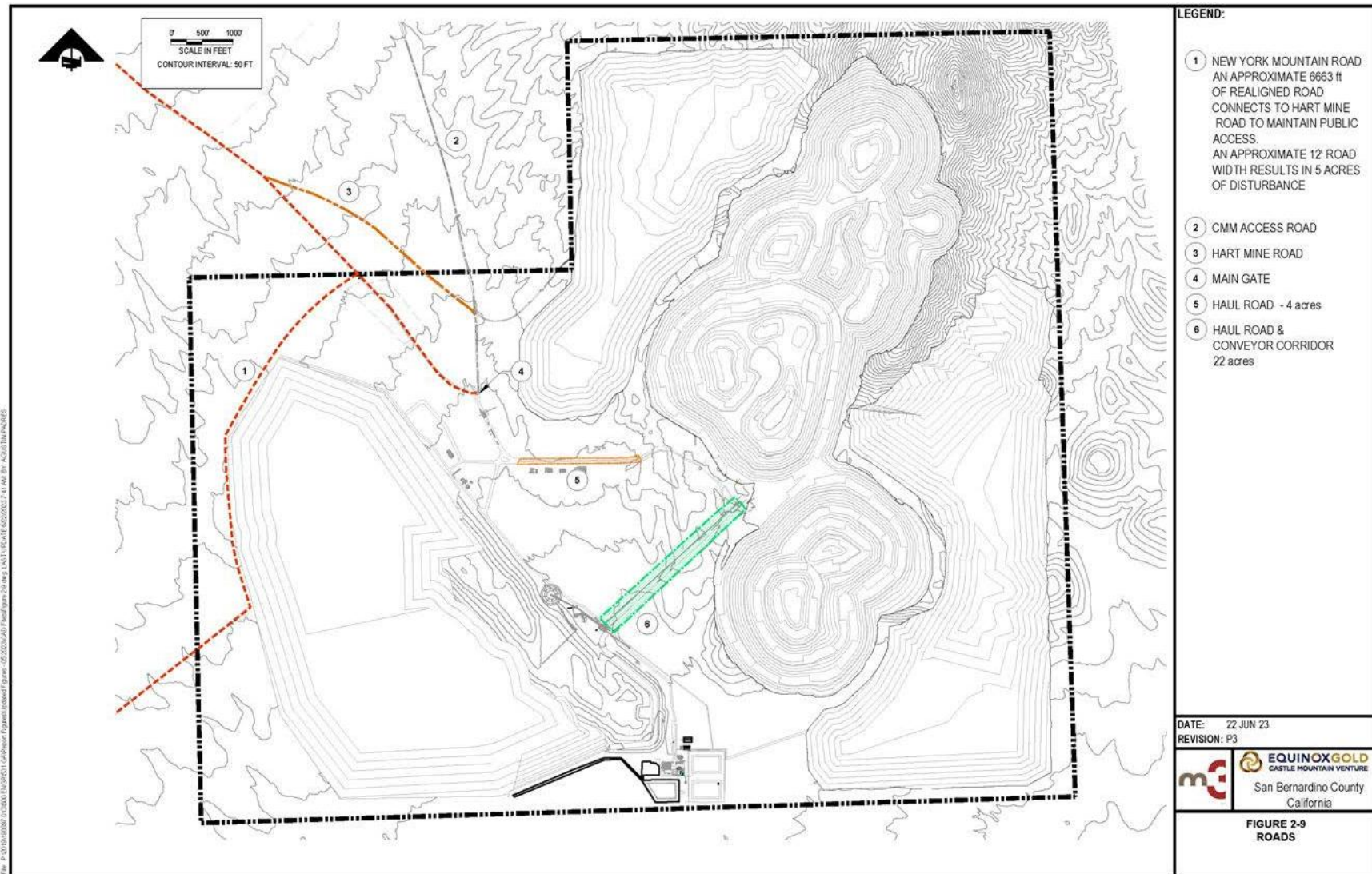
Figure 4.15-4. New York Mountain Road Realignment
