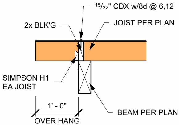
② Joist/Beam Detail
